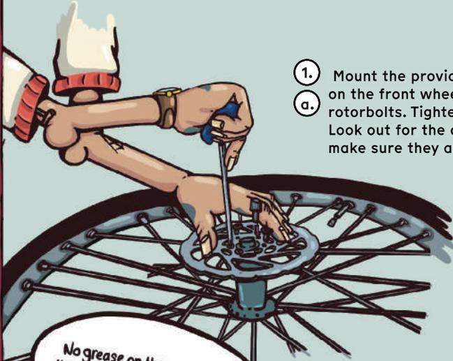
1. Mount the provided 160mm 6 bolt rotor on the front wheel using the 6 torx-25 rotorbolts. Tighten them to 6,2Nm.
