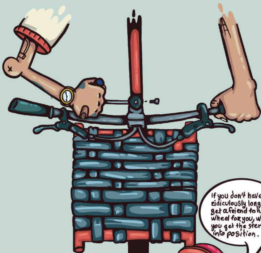
Tighten the top cap to 3-4 Nm, before tightening the stem. Now, align the stem with the front wheel, and tighten the stem to the steering rod, tightening the bolts to 5-7 Nm.
