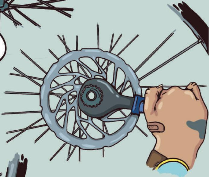
1. Mount the 160mm centerlock rotor on the rear wheel using the locking and the proper tool.
