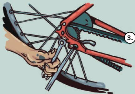
3. When mounting the rear wheel, make sure to have the sliding inserts loose which makes it easier to fit the belt on the front and rear sprocket. Remember the fixing washer and make sure the gear arm on the hub is pointing forward. Then tighten the nuts to 30-45Nm with your 15mm wrench.
