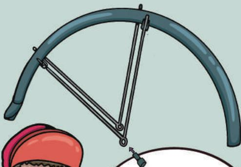
**Don't forget to take out the wheels before you install the mudguards. Or it just ain't happening! Once installed, put the wheels back on to adjust the mudguards.**
