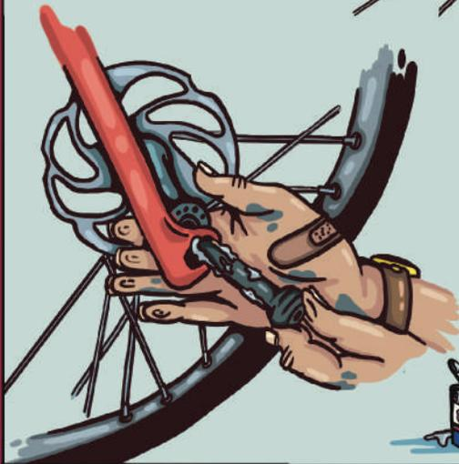
2. Remove the protective plastic inserts from the brake calipers. Mount the front wheel first, and make sure to grease the thru axle. Tighten the axle to 10 Nm maximum using a 6mm allen key.
