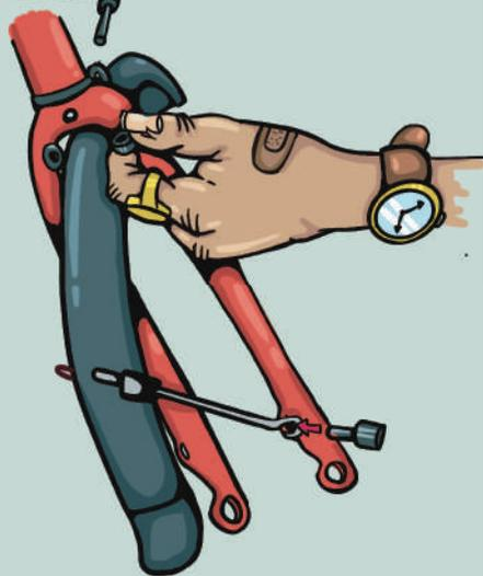
Attach the two straight stays to the front mudguard using the two nuts and bolts provided.
