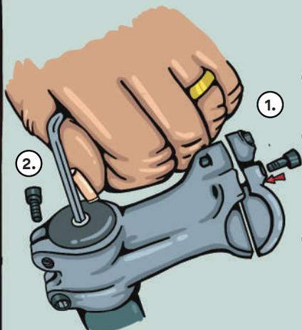
1. Remove the four bolts from the front of the stem, and take off the faceplates.
