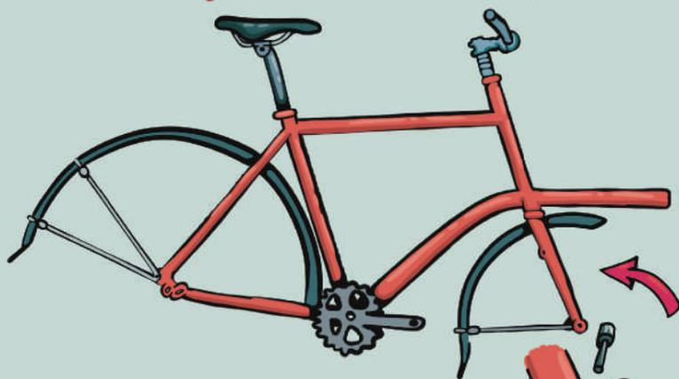
Attach the two V-stays to the rear mudguard using the provided nuts and bolts. Mount the rear mudguards on the bike using the black T25 torx for the V-stays, and the bolts and washers provided in the bag to fasten the mudguards to the rear triangle.
