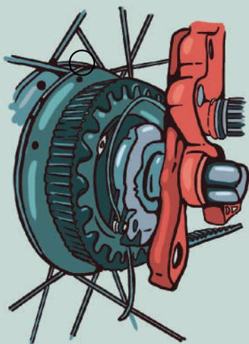
4. Tighten the belt. The easiest way to do this is by using the 15mm wrench and applying pressure on the right hand side nut, which moves the wheel and the sliding inserts back. When the inserts are back and the belt is tight you tighten the inserts with your 6mm allen key.
