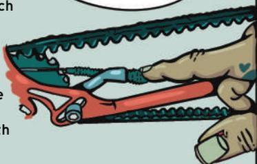
5. Mounting the gear cable. Pull the outer cable towards the rear to give you something to work with. Cable needs to be mounted in the small hook at the back of the hub and the outer cable is mounted in the arm. It might take some bit of fiddling.
